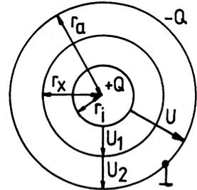
$$\text{Zu 1.2 } U_1 = \frac{\ln \frac{(6+2)\text{cm}}{2 \cdot 2\text{cm}}}{\ln \frac{6\text{cm}}{2\text{cm}}} \cdot U = \frac{\ln 2}{\ln 3} \cdot 10\text{kV}$$
